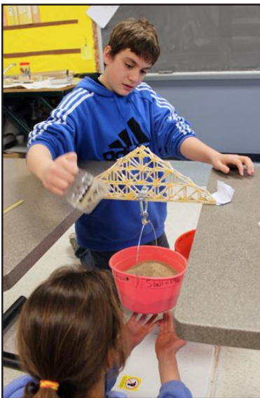
How much sand can the bucket hold before the bridge collapses? Joel G. and Julia S. test their bridge design in one of Mark Wiersma's eighth-grade science projects.
